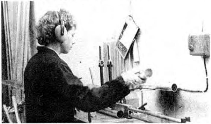
A high speed tungsten saw cuts component parts for Trilite at Optikinetics new production unit in Huntingdon.
